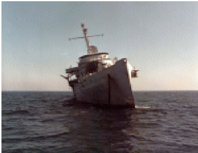
The Ozark with a twelve degree Starboard list due to flooding of three forward decks from the maverick missile explosion
